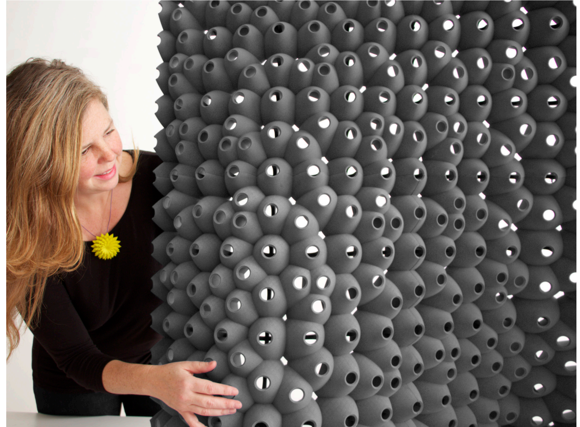
3D printed prototype of building facade
