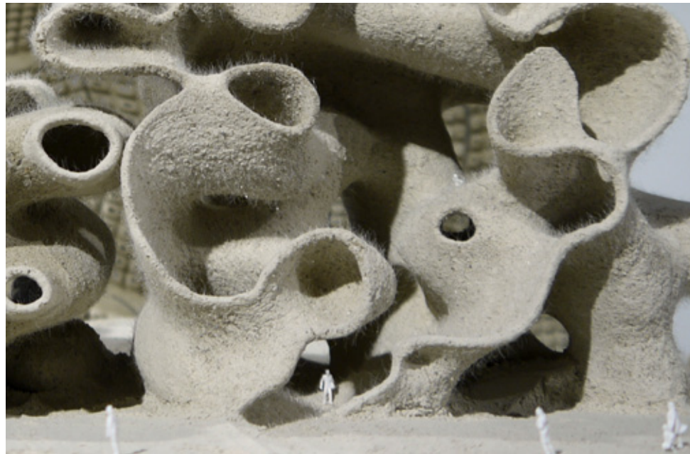
below: 3D printed sand structure right: Tower printed in 4 pieces and stacked together at interlocking sections
